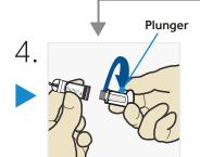
Twist plunger counter-clockwise to loosen and remove.
